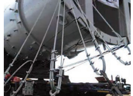
Wire lashing arrangements offer extra insurance against cargo movement.
