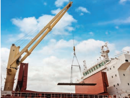
A single, heavy-lift derrick on a cargo vessel poses limitations on the lifting of long columns.
