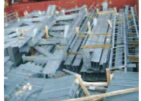
Full cargo hold with inadequate dunnage, showing little regard to the weight imposed on the lower tiers
